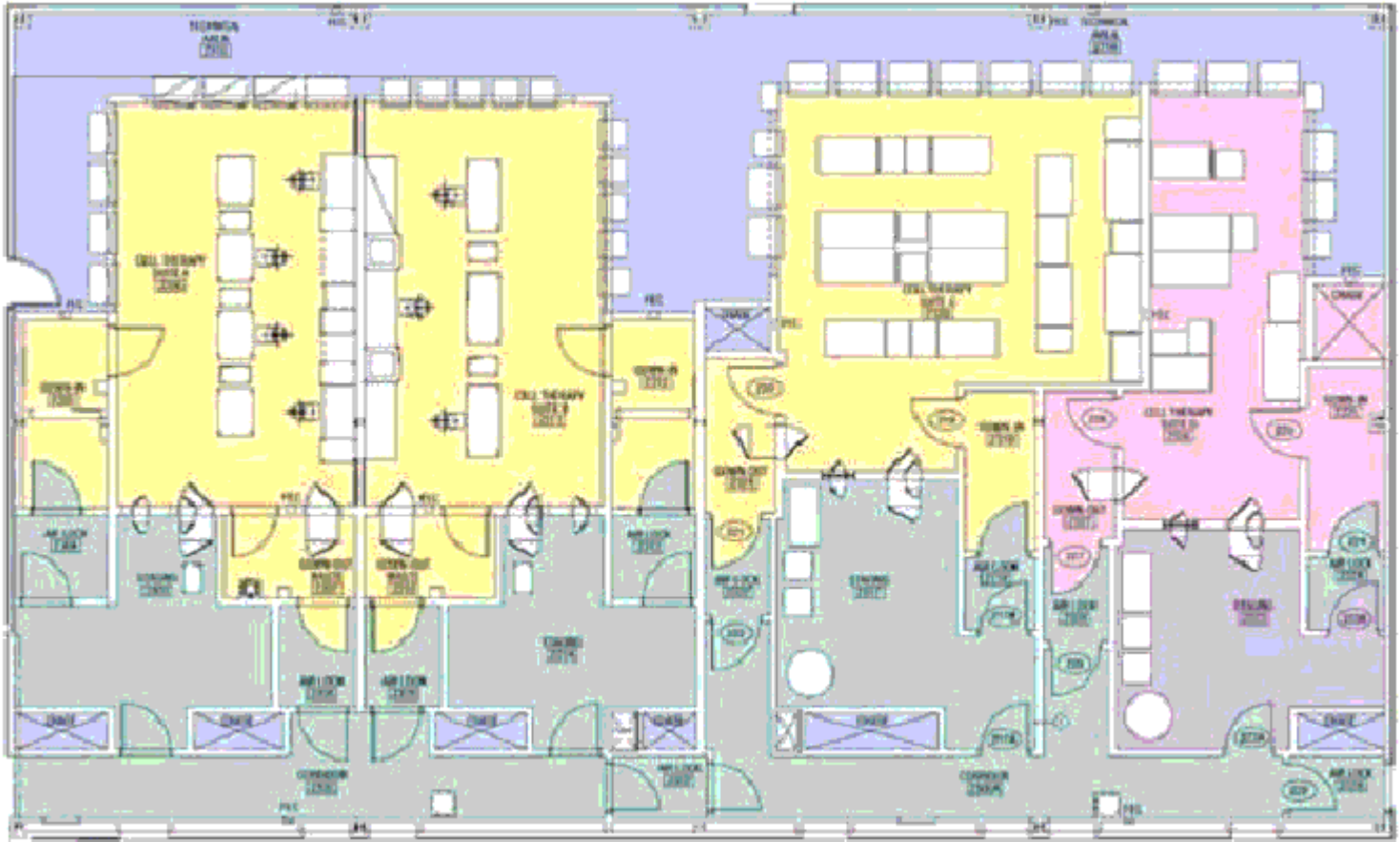
Figure 13. Cell therapy suites at Lonza Walkersville, Inc. The most recent addition to the Walkersville facility includes these 4 suites including 3 class 10,000 suites and a single class B suite. There is more than 2,800 square feet of classified space in this addition
